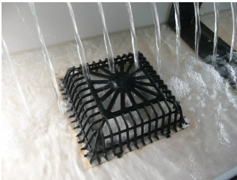
Figure 16.9: Syfon Systems Siphonic Outlet (Rated at 15 L/s), Fitted with Plastic Leafguard
