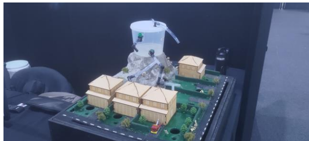
7 - A 'mini' model of the larger laboratory physical model.
