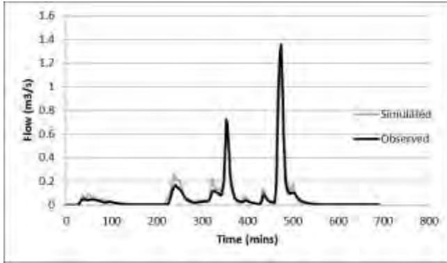
Figure C 9 – Comparison of the observed and simulated flows for Paddocks event V4
