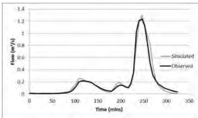
Figure B 8 – Comparison of the observed and simulated flows for event Cal5 (Frederick Street)
