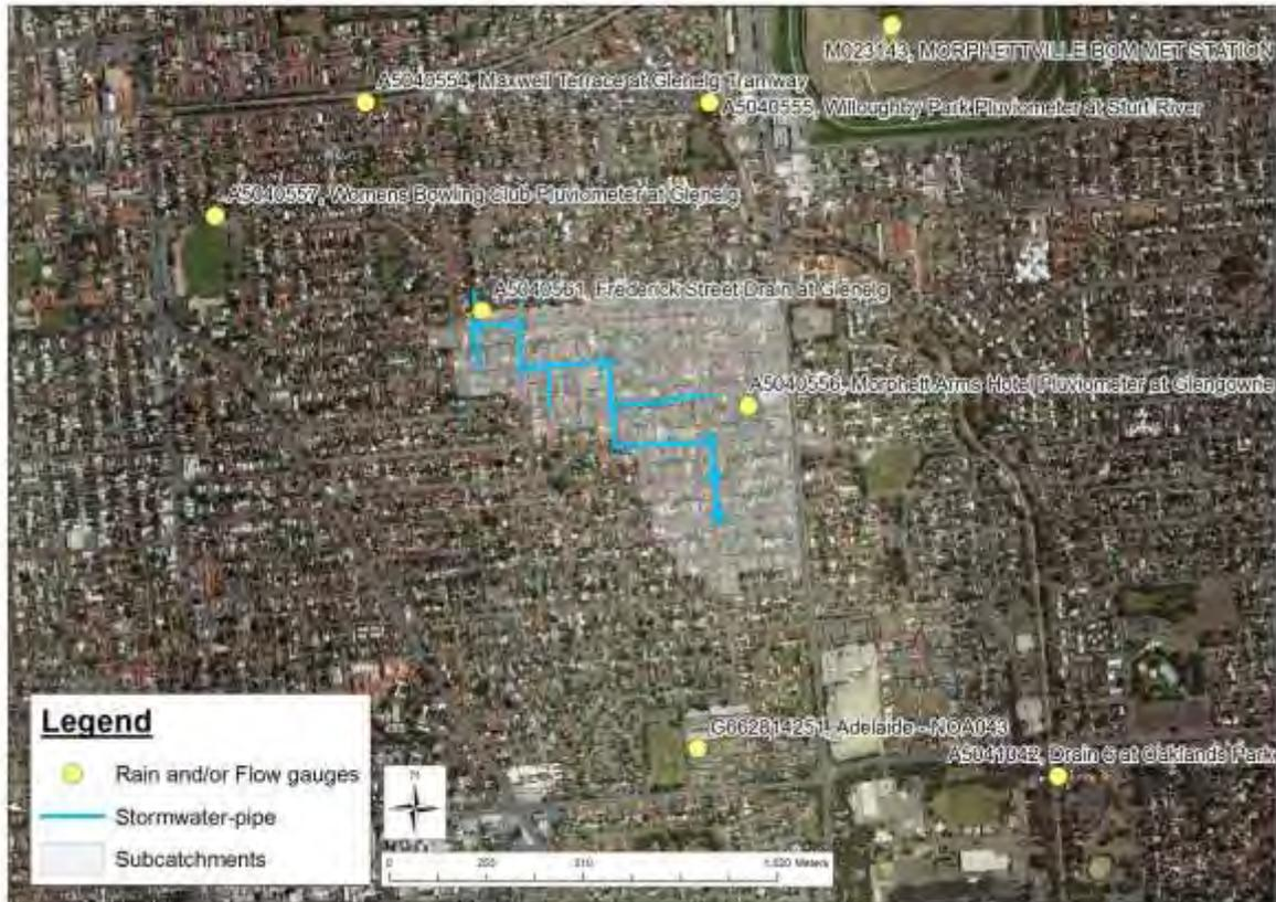
Figure B 3 – Location of gauging stations within and near the Frederick Street catchment
