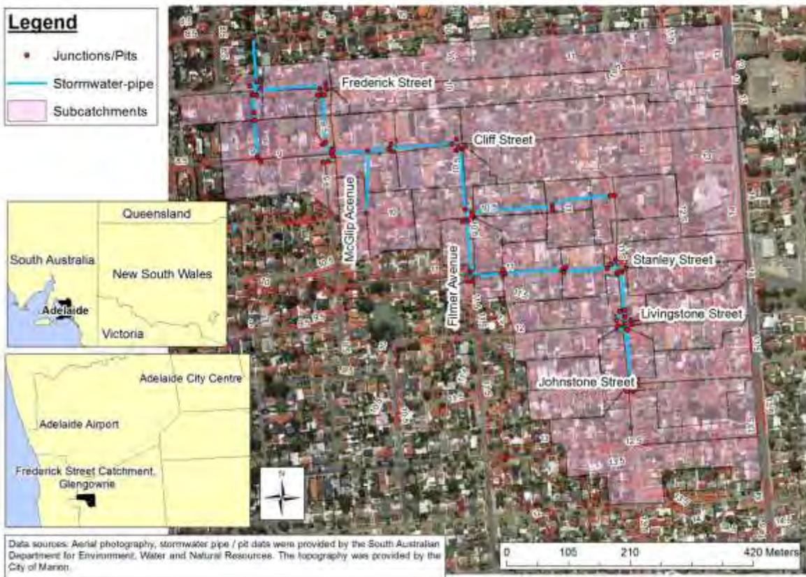
Figure 1 - Location of the Frederick Street catchment in Adelaide, South Australia indicating the catchment area, drainage system layout and roads.
