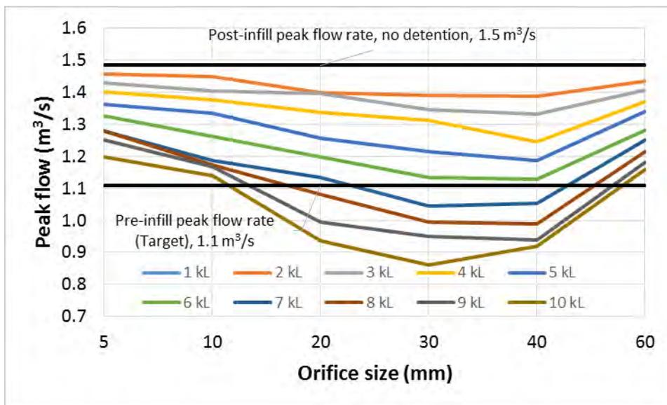
Figure 19 – 50% AEP continuous simulation peak flow estimate for the pre-infill and redeveloped Frederick Street catchment indicating the effect of redevelopment with **detention based storage fitted at the street scale**
