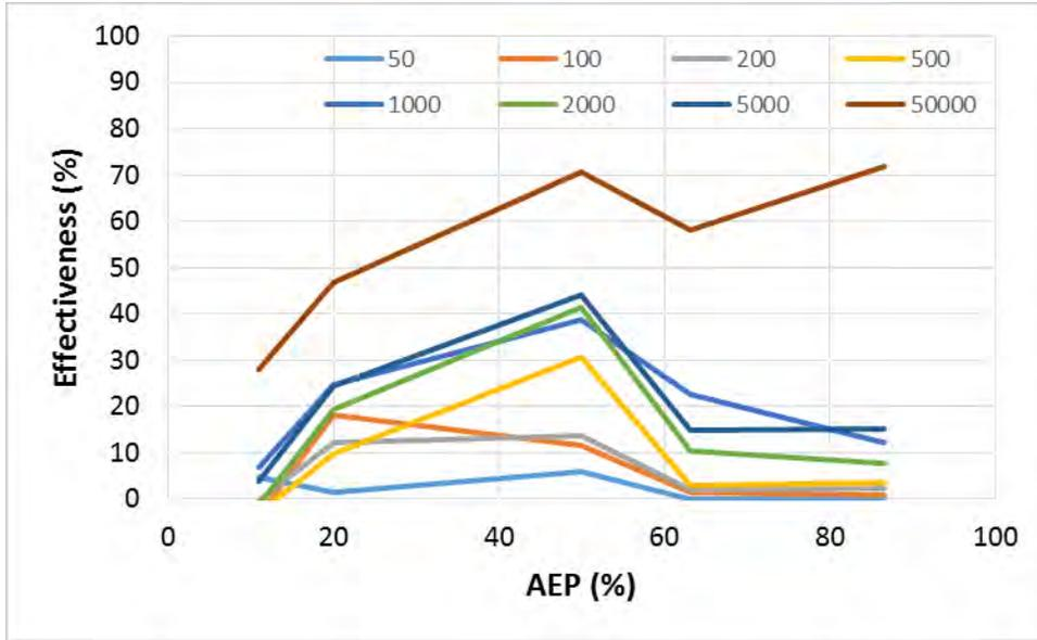
Figure 32 – Comparison of the percentage effectiveness of 5 kL retention tanks (with varying emptying time) to restore ponding volume at a sag point in the Frederick Street catchment with respect to ponding frequency, where a high AEP indicates lower intensity rainfall and low AEP indicates higher intensity rainfall.
