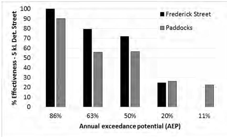
Figure 27 – A comparison of the effect of WSUD Scenario 4 on the Frederick Street and Paddocks catchment, where **lumped detention tanks of 5 kL per redeveloped allotment** were placed at each subcatchment outlet with an emptying time equal to that of a single 5 kL tank per redeveloped allotment with a 20 mm orifice.
