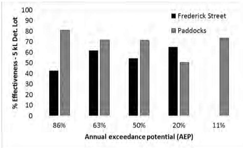
Figure 26 – A comparison of the effect of WSUD Scenario 3 on the Frederick Street and Paddocks catchment, **where 5 kL detention tanks were placed on each redeveloped allotment**, each with an emptying time equal to that provided by a 20 mm orifice.
