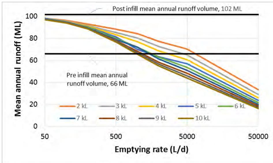
Figure 15 - Mean annual runoff volume (ML) for the pre-infill and redeveloped Frederick Street catchment indicating the effect of redevelopment with a retention based storage fitted in the form of **offsite, lumped retention storages** (note volume is expressed here as a volume per redeveloped allotment in each sub-catchment).
