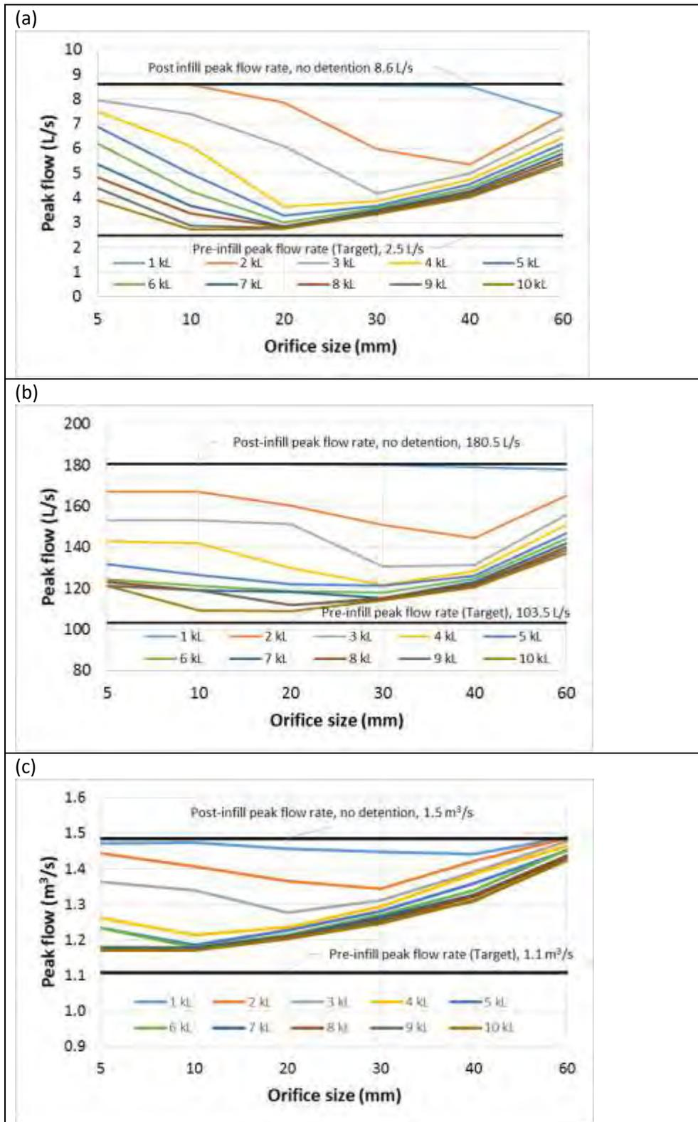
Figure 36 – Comparison of the influence of detention on the 50% AEP peak flow rate from a catchment when simulation of a redeveloped site is undertaken at the (a) allotment (b) street and (c) catchment scale.
