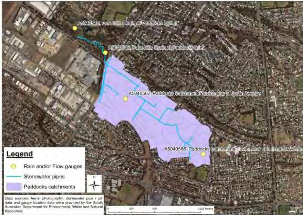
Figure C 2 – Location of gauging stations within and near the Paddocks catchment
