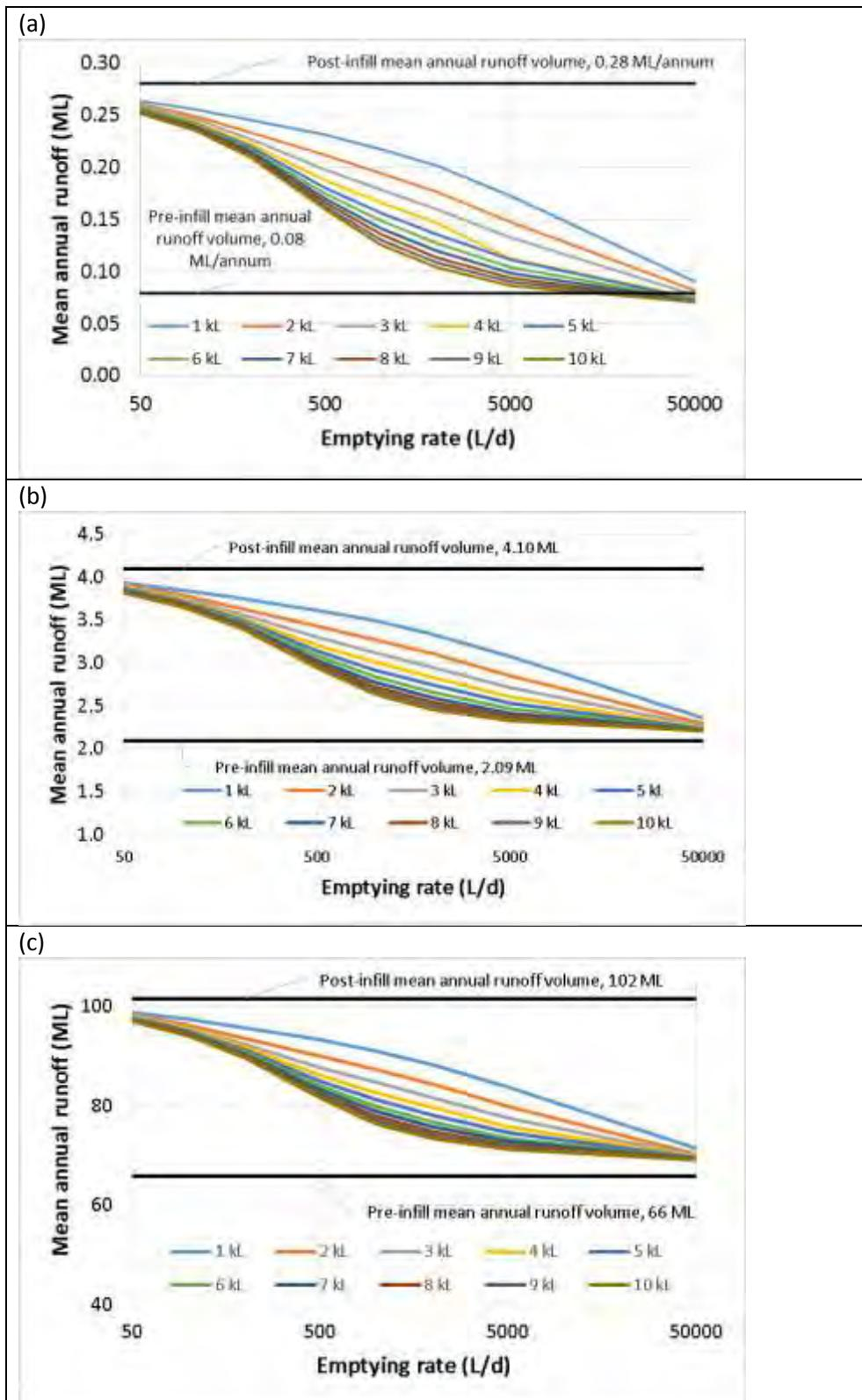
Figure 34 – Comparison of the influence of on-site retention on mean annual runoff volume when simulation of a redeveloped site is undertaken at the (a) allotment (b) street and (c) catchment scale.
