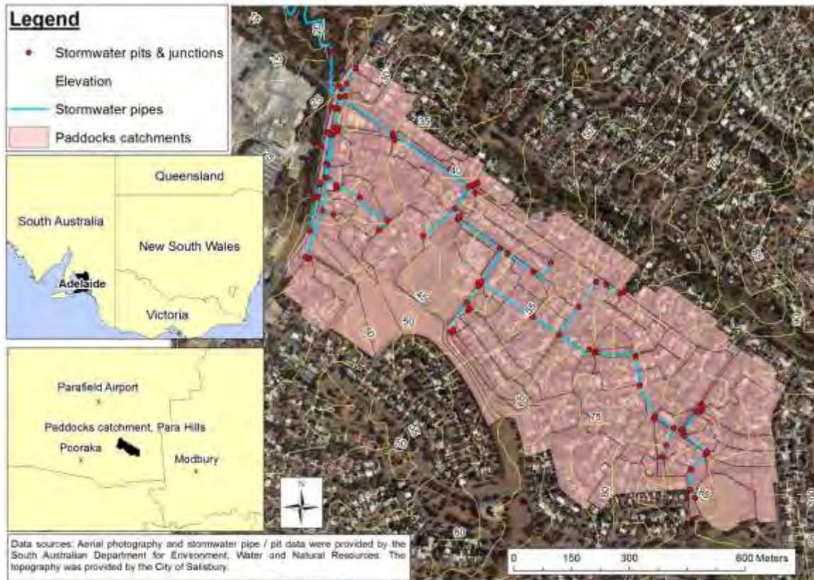
Figure 10 - Location of the Paddocks catchment model, indicating catchment boundary, drainage system layout and surrounding suburbs
