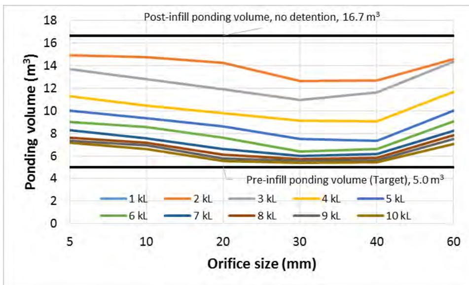
Figure 23 - 50% AEP continuous simulation ponding volume estimate for a sag point in the pre-infill and redeveloped Frederick Street catchment indicating the effect of redevelopment with **detention based storage fitted at the street level**
