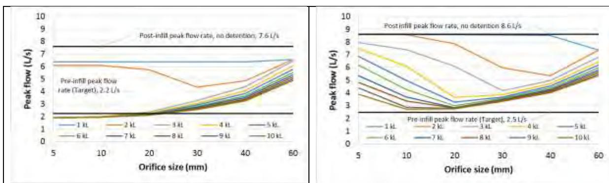
Figure 38 – The 50% AEP peak flow rate from a pre infill, post infill and post-infill with **detention based WSUD at the home allotment**, comparing the results of estimation using a 50% AEP design storm (left) and estimation based on partial series analysis of the continuous flow records
