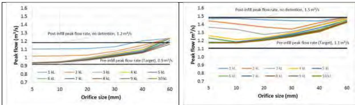
Figure 40 – The 50% AEP peak flow rate from a pre infill, post infill and post-infill with detention based WSUD at the home allotment, comparing the results of estimation using a 50% AEP design storm (left) and estimation based on partial series analysis of the continuous flow records
