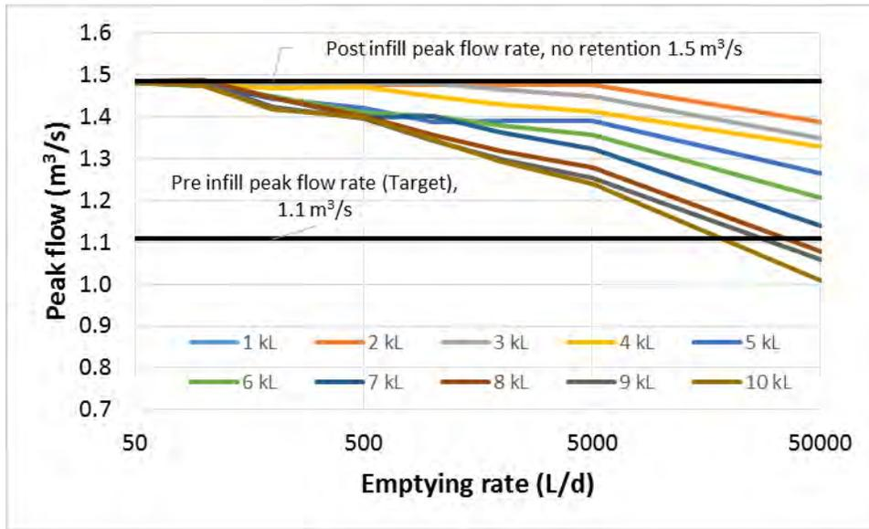
Figure 18 –50% AEP continuous simulation peak flow estimate for the pre-infill and redeveloped Frederick Street catchment indicating the effect of redevelopment with **retention based storage fitted at the street scale**
