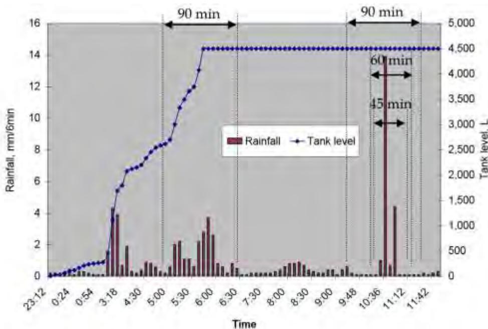
Figure 11 - Continuous simulation results highlighting the storage of a rainwater tank as two rain bursts with a 5 year ARI occurrence on 27/12/1929 Source: Pezzaniti (2003)
