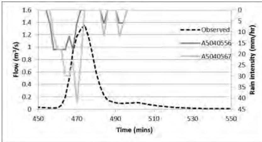
Figure C 10 – Excerpt of event V4, showing the suspicious cessation of rainfall at one gauge
