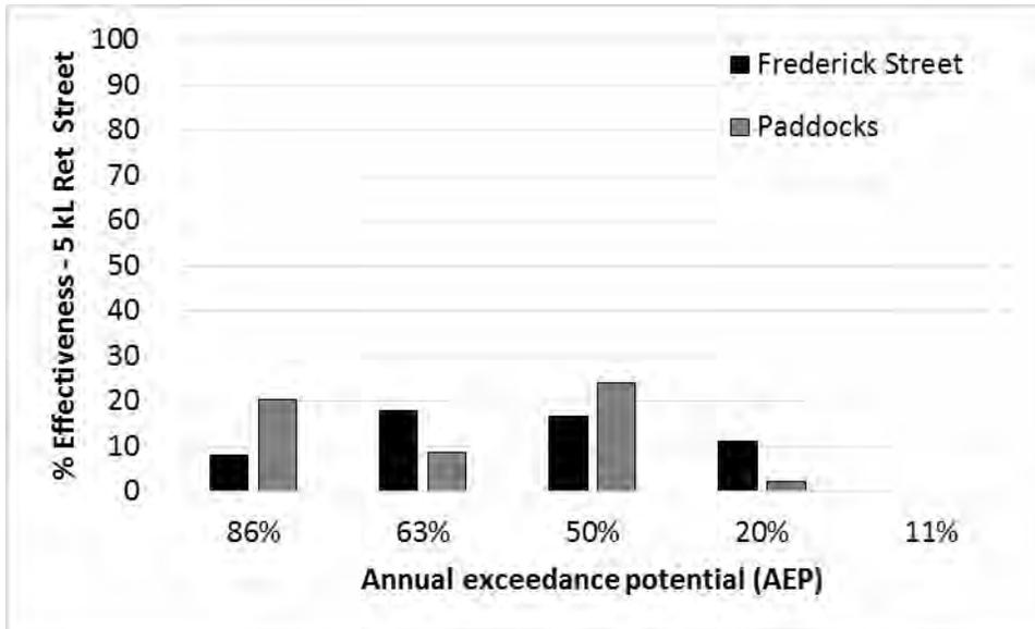
Figure 25 – A comparison of the effect of WSUD Scenario 2 on the Frederick Street and Paddocks catchment, where **lumped retention tanks of 5 kL per redeveloped allotment** were placed at each subcatchment outlet with 500 L/day reuse per allotment.
