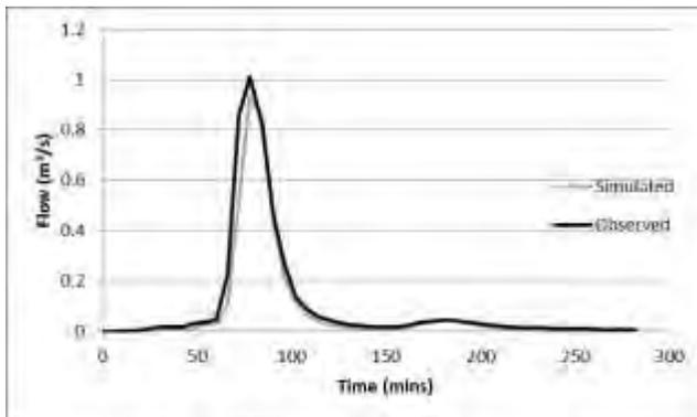
Figure B 10 – Comparison of the observed and simulated flows for event V4 (Frederick Street)
