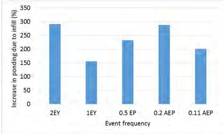
Figure 31 - Comparing the influence of runoff frequency (and rainfall intensity) on the percentage increase in flooding at one sag point of due to infill development in the Frederick Street catchment
