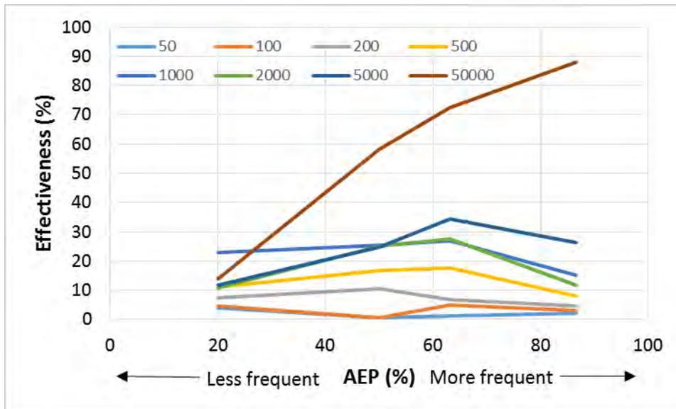
Figure 29 – Comparison of the **percentage effectiveness of 5 kL retention tanks** (with varying reuse) to maintain peak flow rates in the Frederick Street catchment with respect to flow frequency, where high AEP indicates lower intensity rainfall and low AEP indicates high intensity rainfall.
