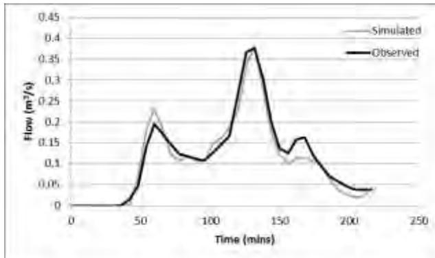
Figure B 7 – Comparison of the observed and simulated flows for event Cal1 (Frederick Street)
