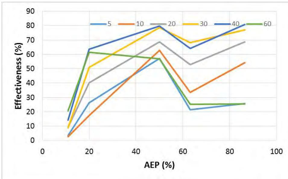
Figure 33 - Comparison of the percentage effectiveness of 5 kL detention tanks (with varying emptying time) to maintain ponding volume at a sag point in the Frederick Street catchment with respect to ponding frequency, where a high AEP indicates lower intensity rainfall and low AEP indicates higher intensity rainfall.
