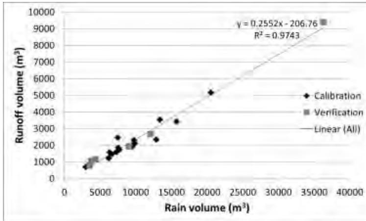
Figure C 5 – Comparison of observed rainfall and runoff volumes for calibration and verification events in the Paddocks catchment
