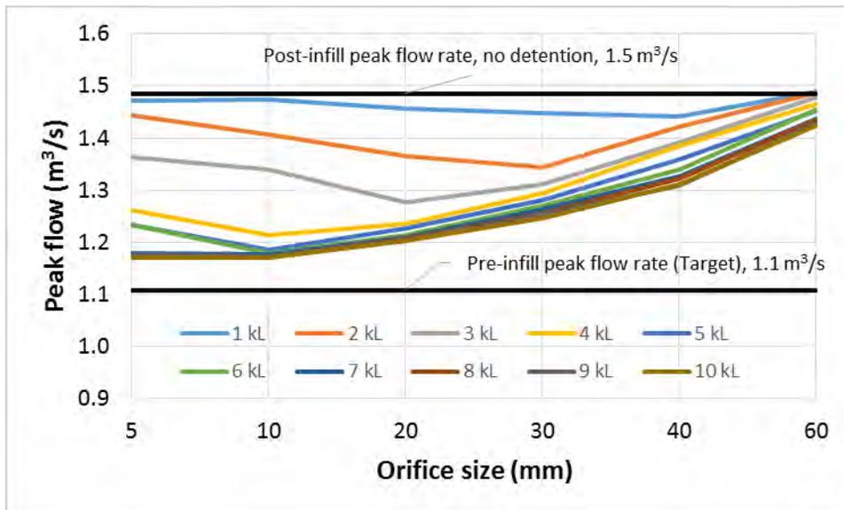
Figure 17 – 50% AEP continuous simulation peak flow estimate for the pre-infill and redeveloped Frederick Street catchment indicating the effect of redevelopment with **detention based storage fitted at the allotment level**
