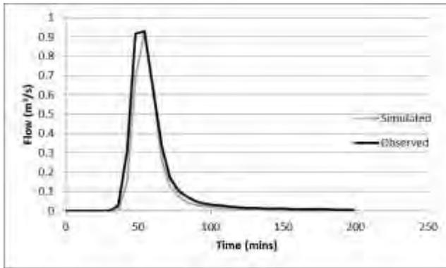
Figure B 9 – Comparison of the observed and simulated flows for event V2 (Frederick Street)
