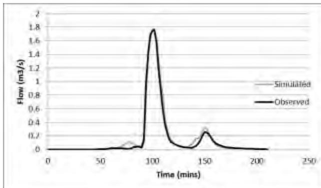
Figure C 8 – Comparison of the observed and simulated flows for Paddocks event V1
