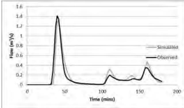
Figure C 6 – Comparison of the observed and simulated flows for Paddocks event Cal 1 (3 October 1992)
