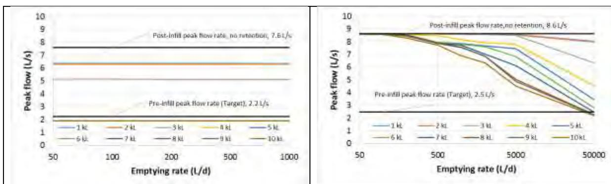
Figure 37 – The 50% AEP peak flow rate from a pre infill, post infill and post-infill with **retention based WSUD at the home allotment**, comparing the results of estimation using a 50% AEP design storm (left) and estimation based on partial series analysis of the continuous flow records
