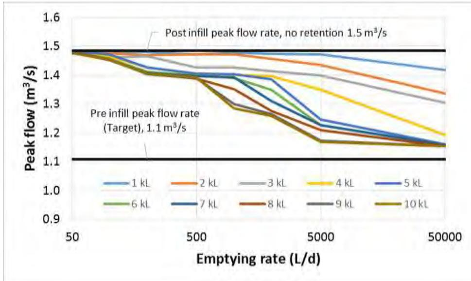
Figure 16 –50% AEP continuous simulation peak flow estimate for the pre-infill and redeveloped Frederick Street catchment indicating the effect of redevelopment with **retention based storage fitted at the allotment level**
