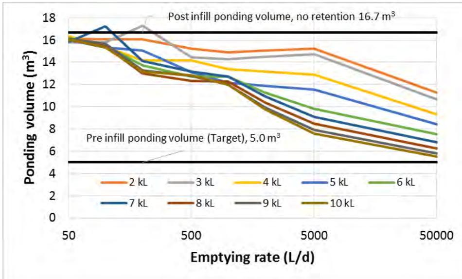
Figure 22 - 50% AEP continuous simulation ponding volume estimate for a sag point in the pre-infill and redeveloped Frederick Street catchment indicating the effect of redevelopment with **retention based storage fitted at the street level**
