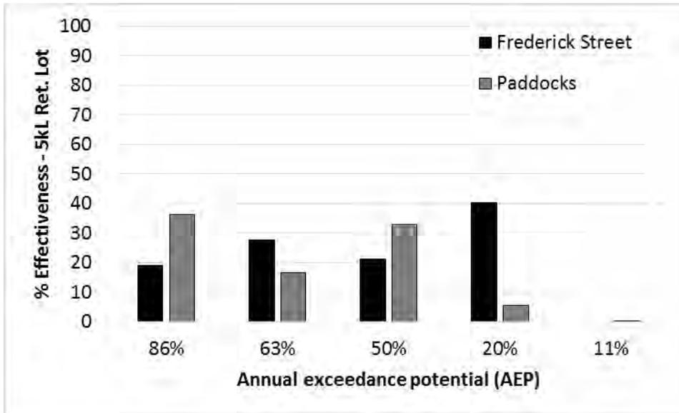
Figure 24 – A comparison of the effect of WSUD Scenario 1 on the Frederick Street and Paddocks catchment, where retention tanks of 5 kL were installed on each redeveloped allotment, with 500 L/day reuse per allotment
