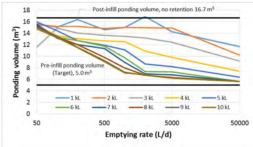
Figure 20 - 50% AEP continuous simulation ponding volume estimate for a sag point in the pre-infill and redeveloped Frederick Street catchment indicating the effect of redevelopment with retention based storage fitted at the allotment level
