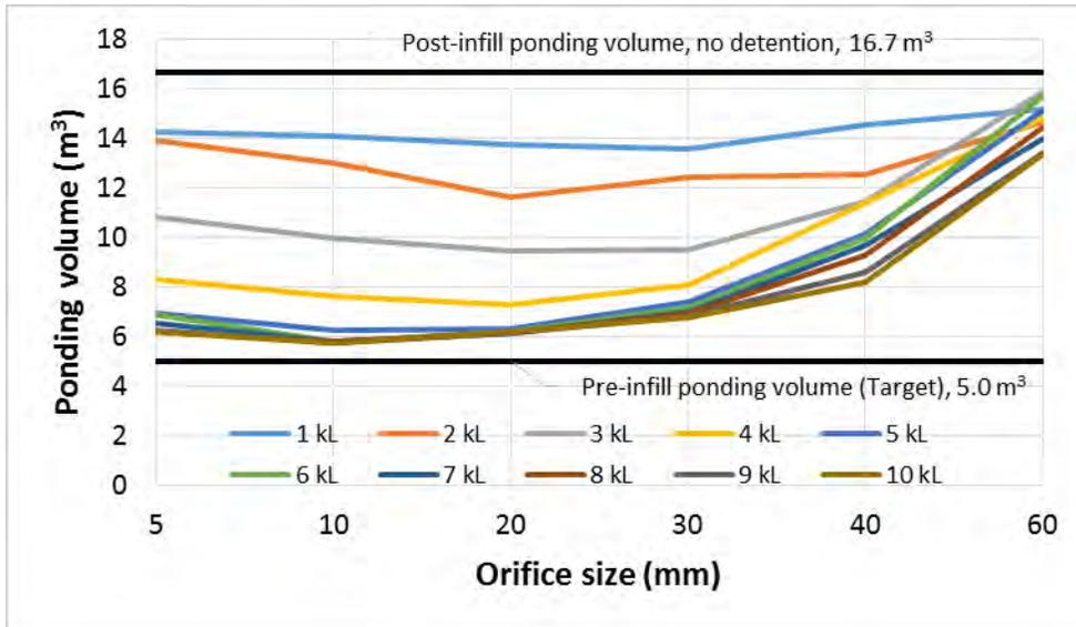
Figure 21 - 50% AEP continuous simulation ponding volume estimate for a sag point in the pre-infill and redeveloped Frederick Street catchment indicating the effect of redevelopment with **detention based storage fitted at the allotment level**
