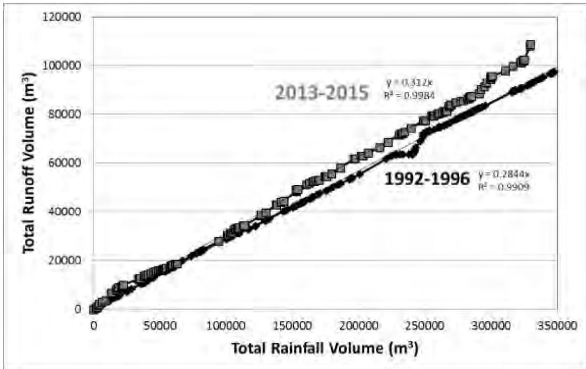
Figure 13 – Comparison of the volumetric runoff coefficient for storms occurring between August 1992 and November 1996, and August 2013 and April 2015
