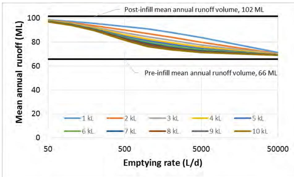
Figure 14 – Mean annual runoff volume (ML) for the pre-infill and redeveloped Frederick Street catchment indicating the effect of redevelopment with a retention based storage fitted in the form of onsite retention systems on redeveloped allotments
