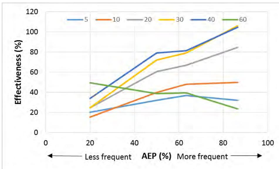
Figure 30 – Comparison of the **percentage effectiveness of 5 kL detention tanks** (with varying emptying time) to maintain peak flow rates in the Frederick Street catchment with respect to flow frequency, where high AEP indicates lower intensity rainfall and low AEP indicates high intensity rainfall.
