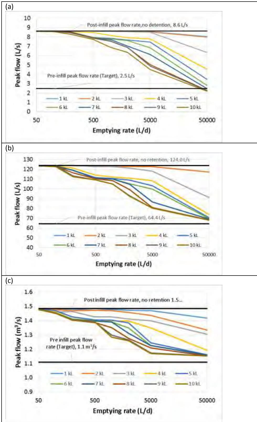
Figure 35 – Comparison of the influence of retention on the 50% AEP peak flow rate from a catchment when simulation of a redeveloped site is undertaken at the (a) allotment (b) street and (c) catchment scale.
