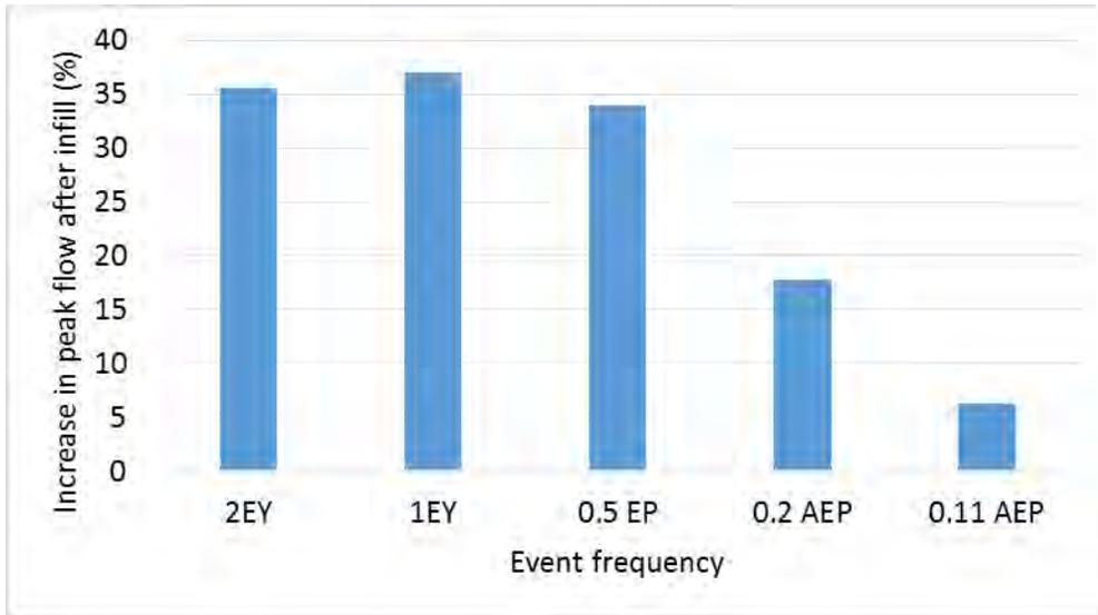
Figure 28 – Comparing the influence of runoff frequency (and rainfall intensity) on the percentage increase in peak flow rate due to infill development in the Frederick Street catchment
