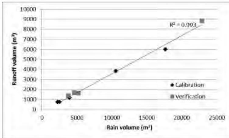
Figure B 6 – Comparison of rainfall volume and runoff volume for the calibration and verification events of the Frederick Street model
