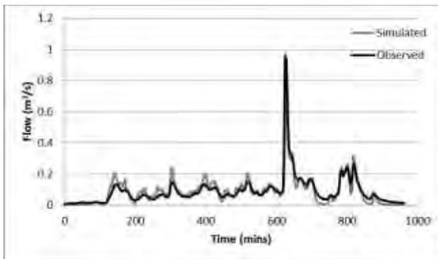
Figure C 7 – Comparison of the observed and simulated flows for Paddocks event Cal 2 (8 October 1992, #1)
