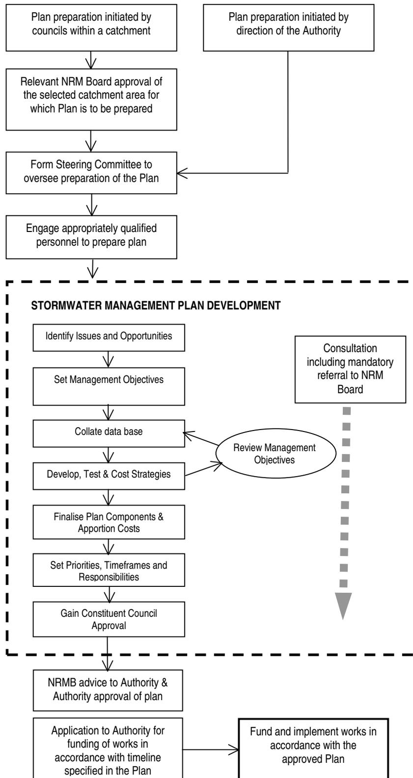
Figure 3.1 Stormwater Management Plan Preparation Process
